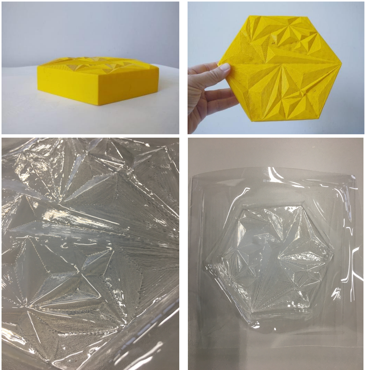
Figure 8: 3D printed mold for vacuumforming and the mold of PETG. Source: image from the author
