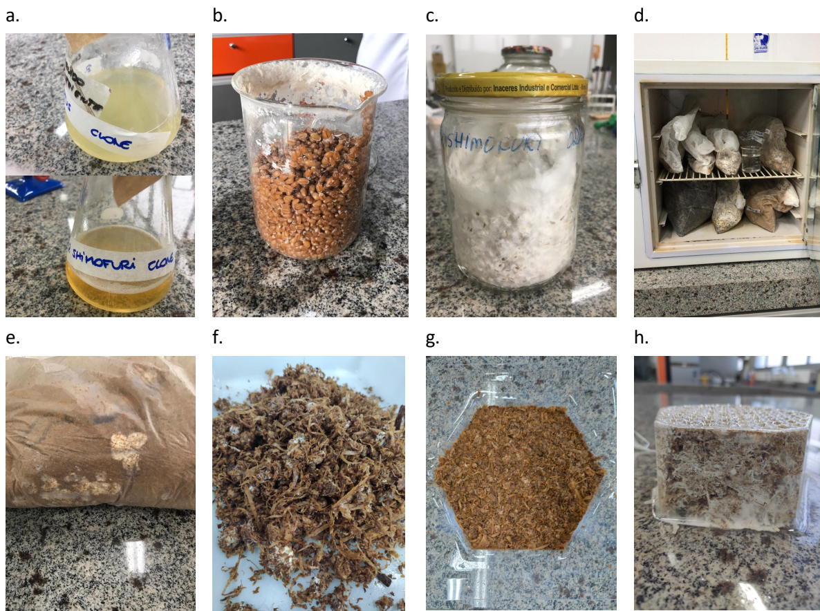
Figure 10: Stages of the composites manufacturing process up to the moment of research: a. cultivation on nutritious substrate; b. spawn production; c. spawn colonized with mycelium; d. incubation of inoculated substrates with colonized spawn; e. start of mycelium growth on the substrate; f. pre-colonized substrate; g. transfer of the colonized substrate to the molds; h. intermediate stage of the colonization process in the forms, before dehydration. Source: image from the author
